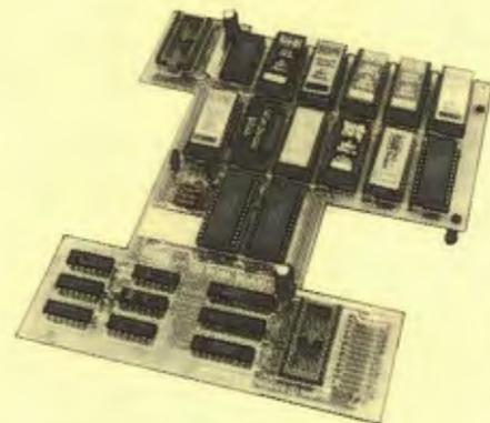
In the May 1986 Micro User's independent review, the writer concludes, "The board has been well laid out. Its position is much better than others - not over the HOT RAM chips and further away from the disc controller area". "I give the solderless ROM board the thumbs up and wish it success".
