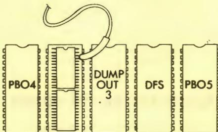
This new unit from Watford, which utilises the latest in Static RAM technology, offers 16k of easy-fit sideways RAM in a very compact unit with a footprint no larger than a standard 28pin EPROM. With only a single flying lead terminating in a mini hook-on probe, to fit, (no soldering required) this compact unit works with any BBC Micro with or without a ROM board. **Compatible with BBC B Plus.** Like our other 16K RAM Modules, this unit is very simple to fit.
