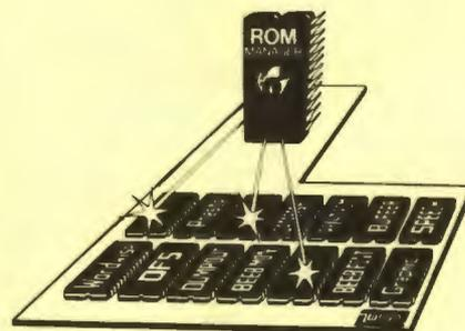
Probably the most powerful way of expanding the BBC micro is from the use of Sideways ROMs. One problem faced by the avid ROM collector is that of ROM command clashes. The solution is very simple in the form of the ROM that "Provides comprehensive management of all your installed ROMs". (Quote from BEEBUG November '84.)
