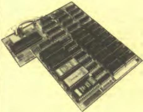
Watford Electronics announced the first ever commercial ROM board for the BBC micro, the Watford Electronics 13 ROM Socket Board 3 years ago. Following the success of this board, we have designed what probably represents the ultimate in expansion boards, the new Watford Electronics ROM/RAM board. This highly versatile and sophisticated board represents the latest in "2nd generation" sideways ROM technology for the BBC micro, designed to satisfy the serious BBC user.
