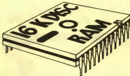
This is the RAM you've been waiting for!! This battery backed up, write protectable 16K sideways RAM board allows you to run from disk every sideways ROM available. Beware of other sideways RAM boards which are not backed up as certain ROMs will not run in these boards even though the RAM can be write protected. The Battery Backup facility allows retention of DATA after power off. On switch on the Micro will think the WATFORD DISC RAM is a ROM. Features available are:
